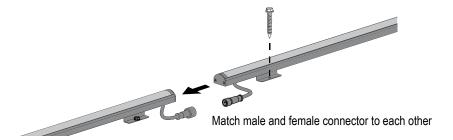
Connect male and female connectors. Make sure to screw female connector to male connector tightly to prevent water from getting into the connectors. Attach end cap connector to the end of run.
